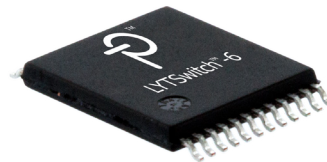
Figure 2. High Creepage, Safety-Compliant InSOP-24D Package.
